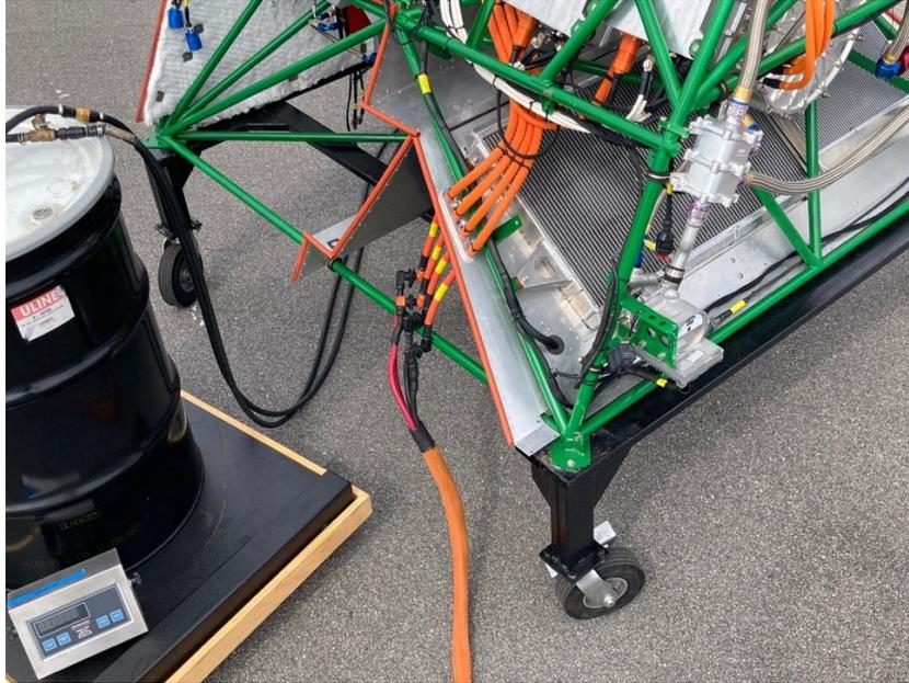
*Direct Measurement of Fuel Consumption and Electrical Output
